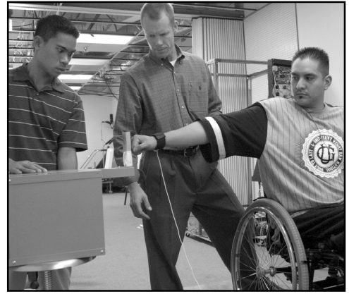
Figure 5. A subject with a spinal cord injury in a wheelchair leaning to the right side at minimal reach to measure stability.
