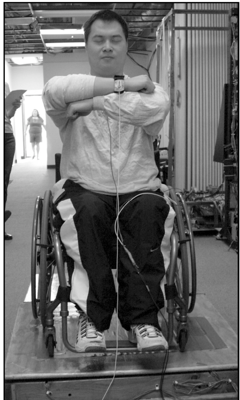
Figure 3. A subject in a wheelchair on the balance platform with eyes closed to measure seating stability.
