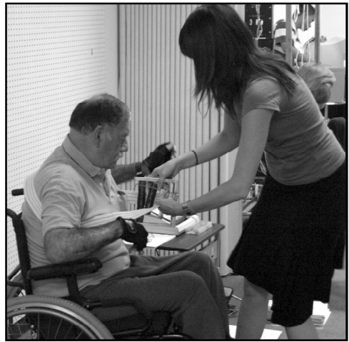
Figure 2. Strength is measured in a wheelchair bound subject during extension of the back muscles. In practice, the subject would bend 30 degrees forward and then try to straighten up. An isometric strain gage transducer was used to measure the strength.
